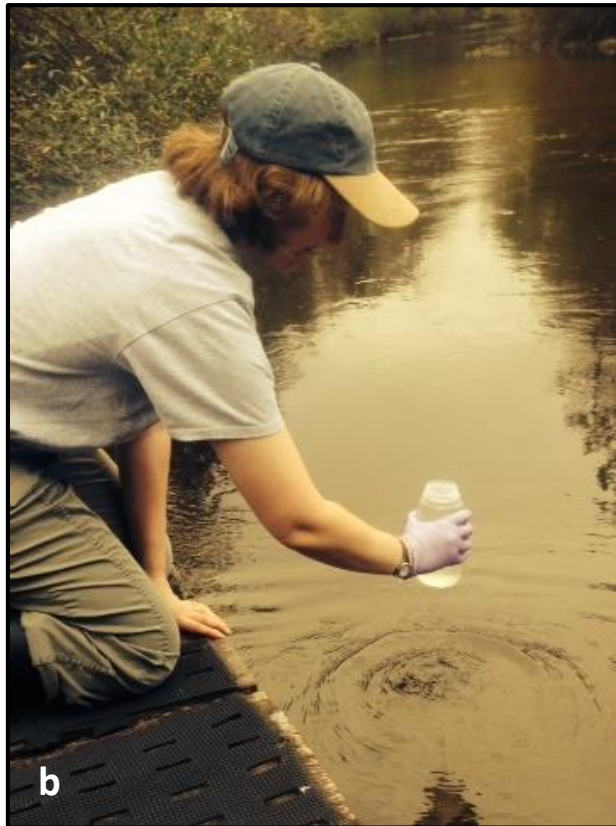
Figure 8. Collect water in (a) disposable Whirl-Pak® bag or (b) sterile Nalgene bottle.
