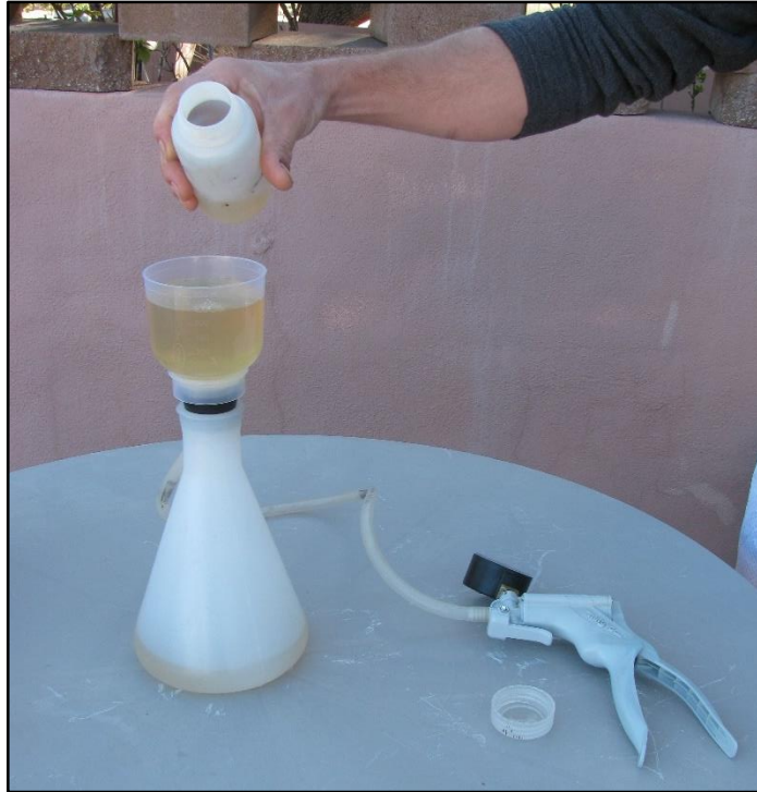
Figure 9. Pour sample slowly into filter funnel, filling funnel to 250 mL mark.
