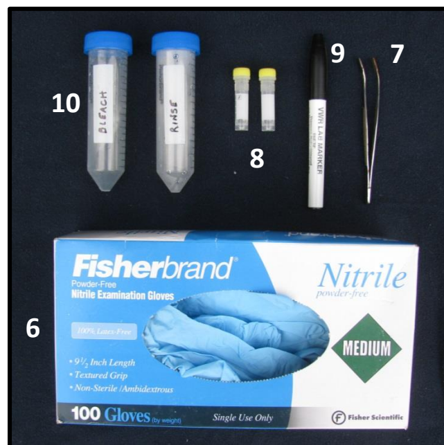
Figure 2. Latex or nitrile gloves (6), forceps (7), 2 mL tubes with 1 mL ethanol (8), ethanol-proof lab marker (9), and 2 50 mL tubes with 50% household bleach solution distilled water (10).
