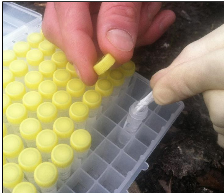
Figure 13. Place filter in 2 mL tube of ethanol.
