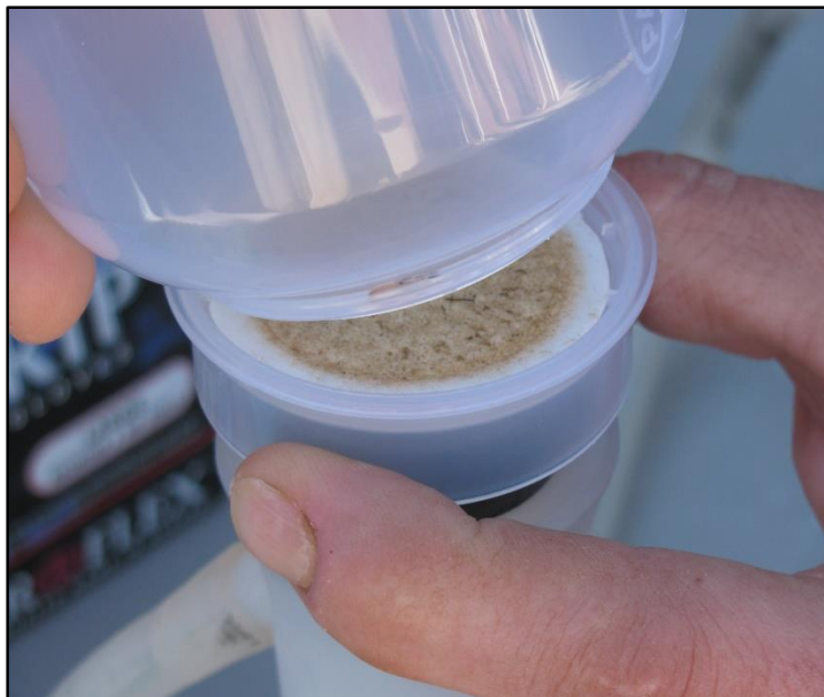
Figure 11. Remove funnel cup.
