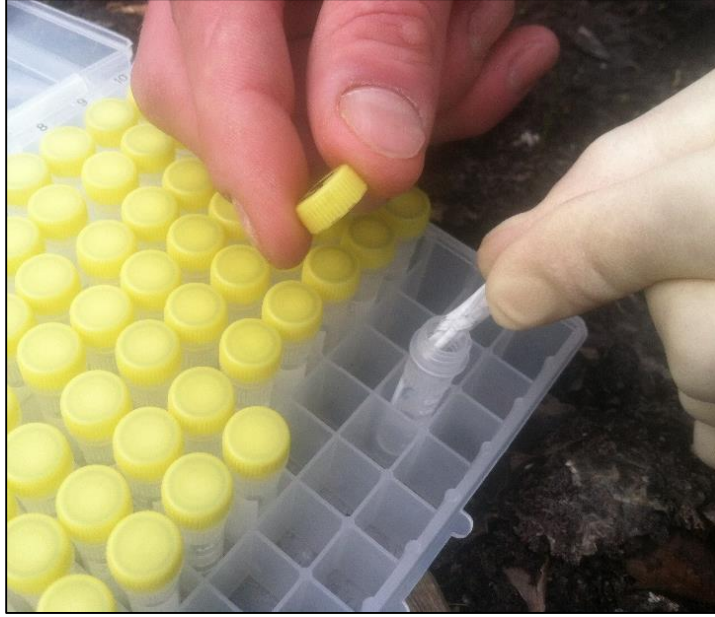
Figure 13. Place filter in 2 mL tube of ethanol.
