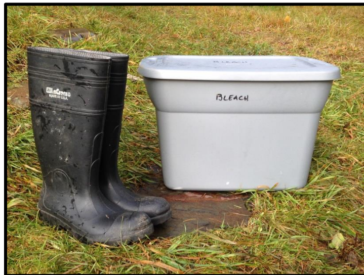
Figure 6. Clean boots thoroughly between sites. Decontaminate with 10% bleach and rinse well with tap water.
