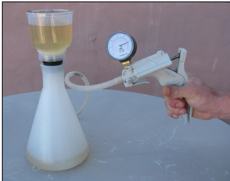
Figure 10. Engage hand pump to begin filtration.
