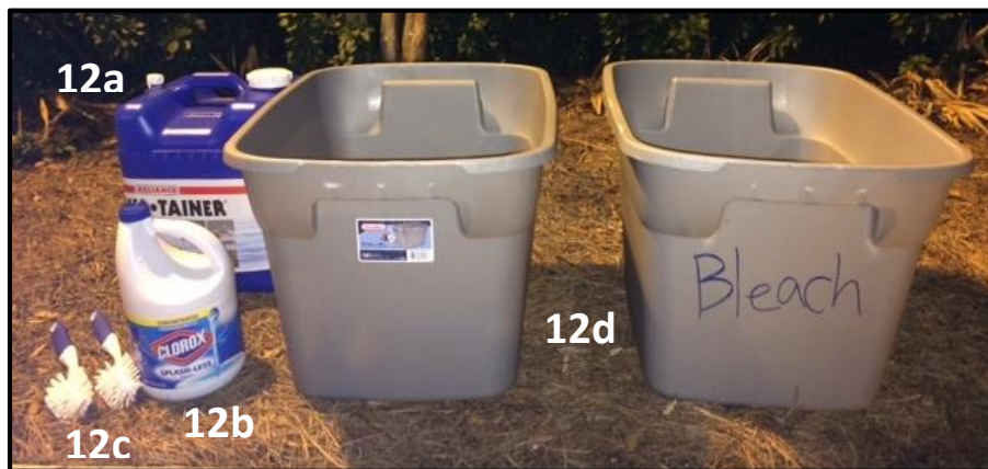
Figure 4. Water (12a), bleach (12b), scrub brushes (12c), and tubs (12d) for decontaminating boots and equipment between sites.
