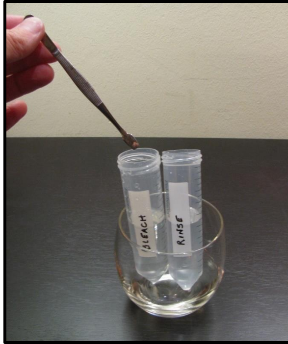
Figure 5. Decontaminate forceps in 50% bleach for at least 1 minute between each sample. Rinse well with distilled water.
