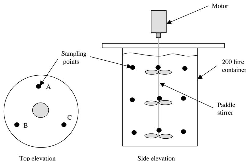
Fig. 1. Schematic of manure sampling device and sampling locations (container dimensions: height = 91 cm; diameter = 56 cm)
