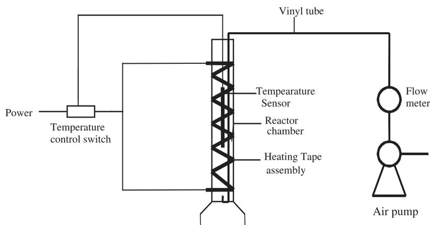
**Figure 1.** A schematic of the equipment and instrumentation used in the experiment.
