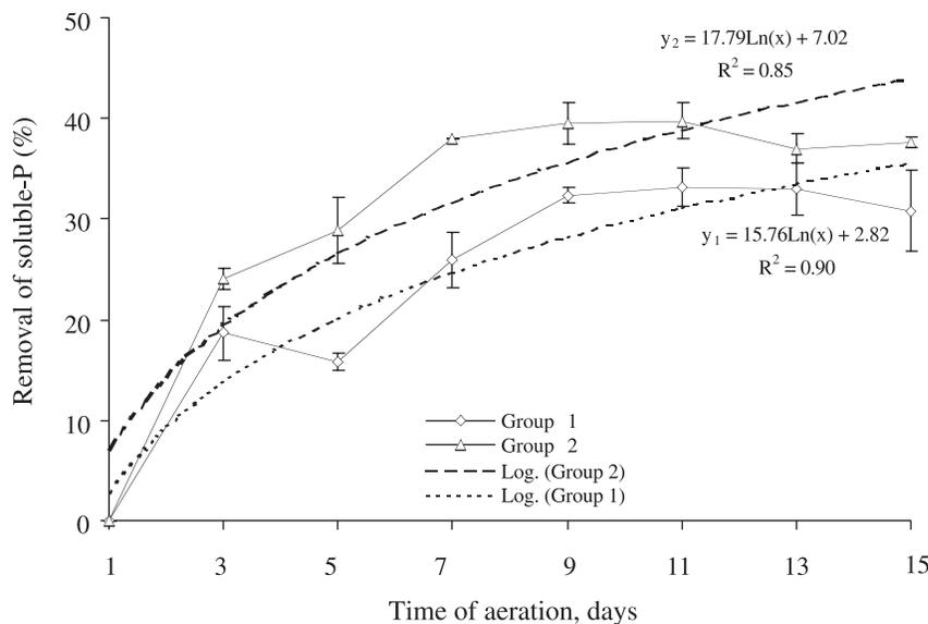
**Figure 3.** Variation of phosphorus removal with aeration time and bioreactor temperature.
