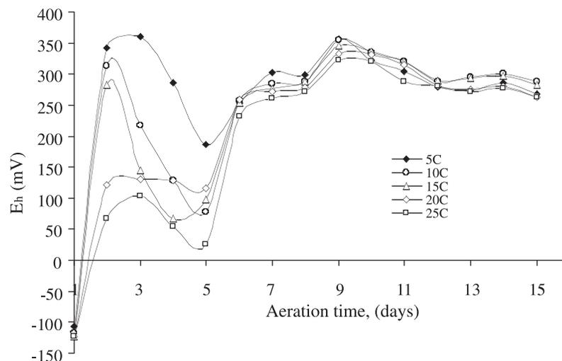
**Figure 2.** Changes in the oxidation–reduction potential of the manure with time and temperature during aeration.
