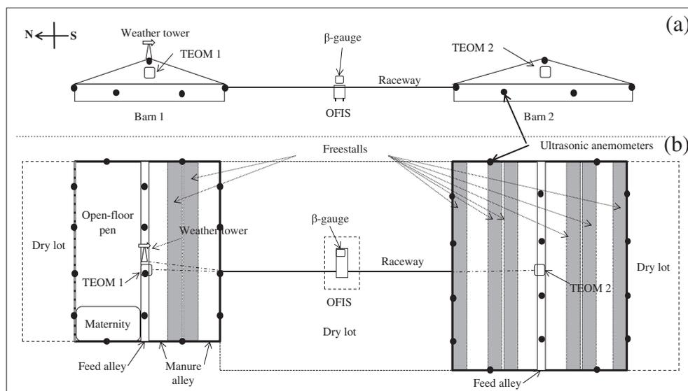
Fig. 1. Layout of the barns, on-farm instrument shelter (OFIS), and monitoring locations: (a) end view; (b) plan view.
