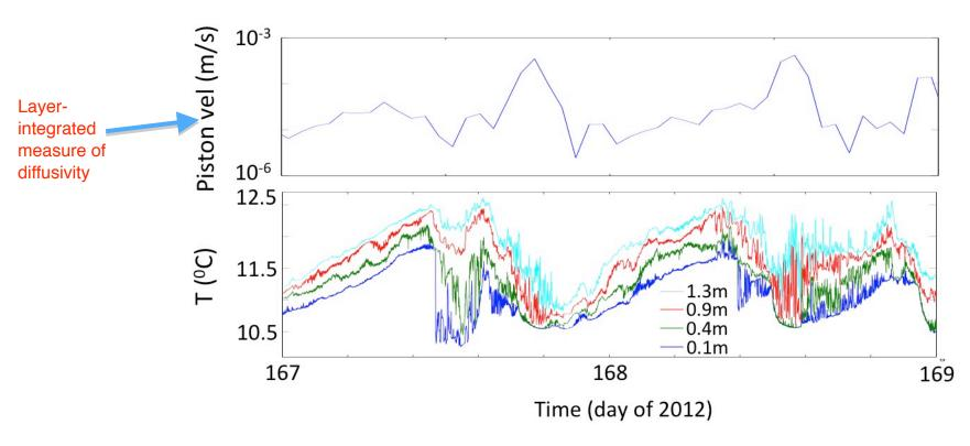
Big variations in near-bed mixing resulting from periodic stratification resulting from internal waves
