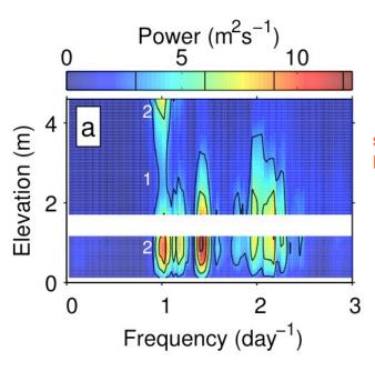
spectra measured by upward- and downward-looking ADCPs Blanked out elevations (1.5-1.8m) span location of ADCP
