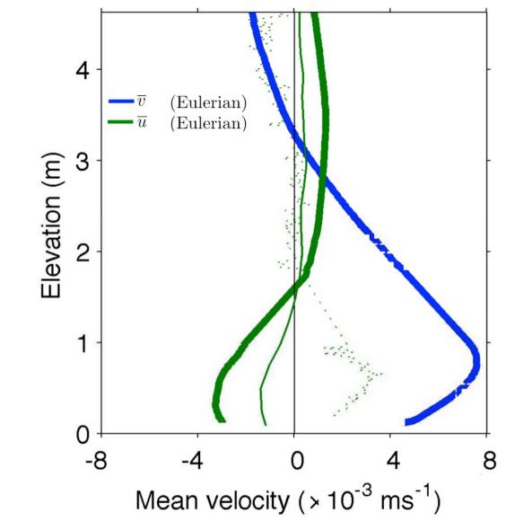
When daily fluctuations associated with waves are averaged out, residual mean is small, with along-lake & downslope boundary layer jet dominant
