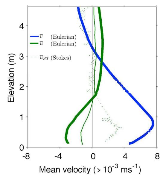
So, despite downslope Eulerian mean velocity, particles might not on average be moving downslope
