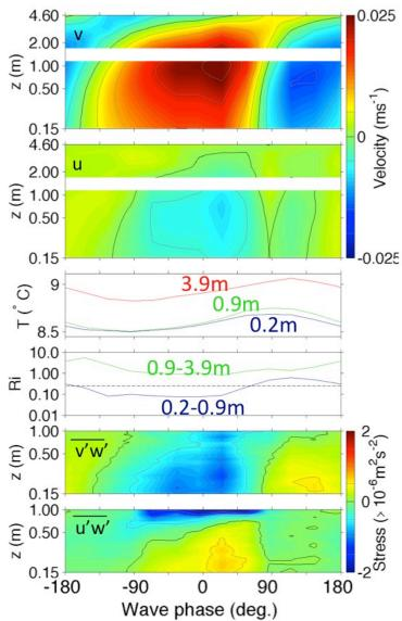
Turbulent Reynolds stress estimated by differencing along-beam velocity variances.
