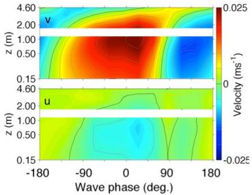
For several weeks of data, every time was associated with a waves phase, with phase varying 360 deg in each (roughly diurnal) wave cycle. Then all data with roughly the same phase averaged, to produce phase averages shown above.
