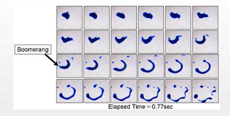
These images exhibit the major characteristics of the surface tension driven "boomerang" like dissolution of a drop of 1-octanol: the crescent-like shape in the beginning, the continued elongation of the droplet, the eventual lack of stability and integrity, and then the lysis.
