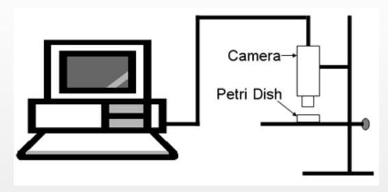
Distilled water was used throughout the experiments. The standard dish that held the water had a diameter of 5.3cm. Other dishes used had diameters of 2.5cm and 6.8cm. A video camera was used to film the experiments. The droplets were hand-dropped or touched to the water surface in volumes ranging from 5-25uL. The videos were recorded at 30 frames per second with a resolution of 720 x 480 pixels. Frame-by-frame analysis of the droplets was done using Scion Image.
