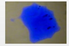
This picture on the right shows what happens when a finger protrudes far enough to overcome the molecular forces holding the drop together. When this occurs the finger "necks down", gets smaller where it is attached to the drop, and, within an average time period of one tenth of a second, separates to become its own drop.
