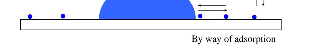
Droplet growth can happen in two ways: directly from the vapor, or via adsorption at the surface. Our equation for droplet growth includes terms for both contributions.
