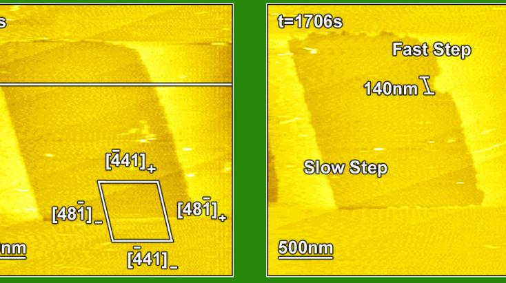
scan is 7.2 nN and the tip speed is 7  $\mu$ m/s in a solution concentration of  $\sigma$  = 1.3. Growth appears to be normal to the fast step as shown in figure on the left
