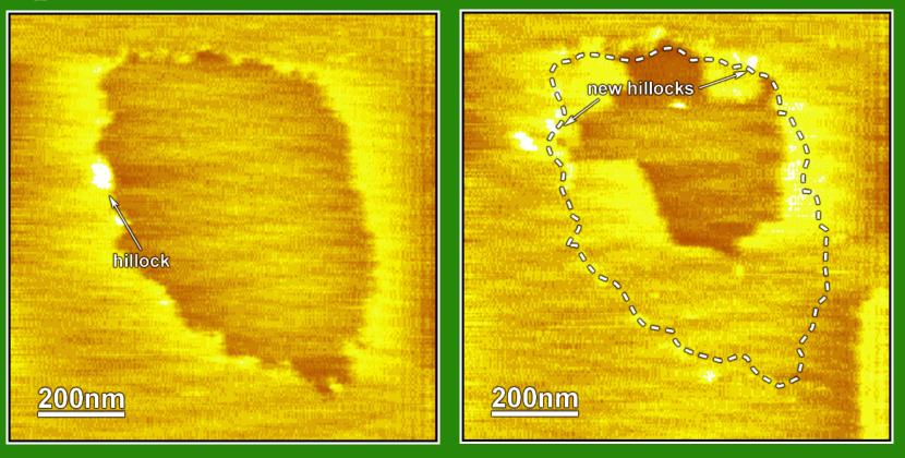
When placed in very supersaturated solution, spontaneous growth occurs and new hillocks form around the boundaries of the old pit. This suggests that rapid growth causes defects which are not observed when the growth is induced. These images were taken at a  $\sigma = 6.9$ .
