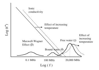
Fig. 3 Frequency and temperature effects of different dispersion mechanisms on loss factor [103]
