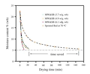
Fig. 1 Microwave and spouted bed combined drying of diced apples at different power level in comparison with spouted bed hot-air drying
