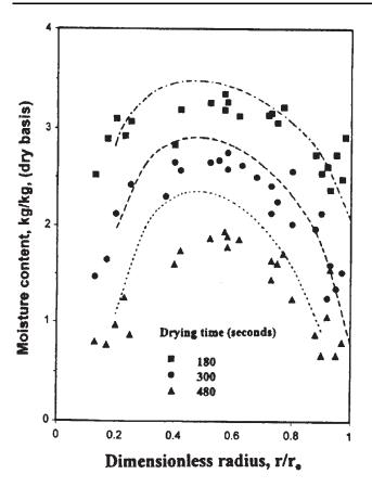
Fig. 6 Comparison between model predicted and experimentally determined moisture distributions [59]
