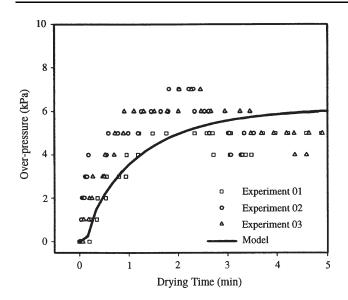
Fig. 7 Over-pressure in microwave-assisted spouted bed drying of diced apples with microwave power of 10 W/g and hot-air temperature of 70  $^{\circ}$ C [37]
