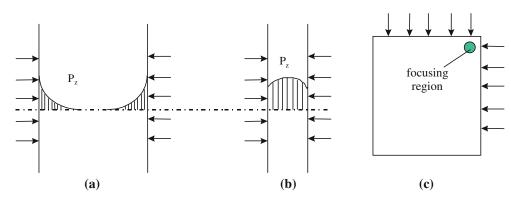
Fig. 4 Microwave power density distribution inside a material. Arrows indicate incident microwaves
