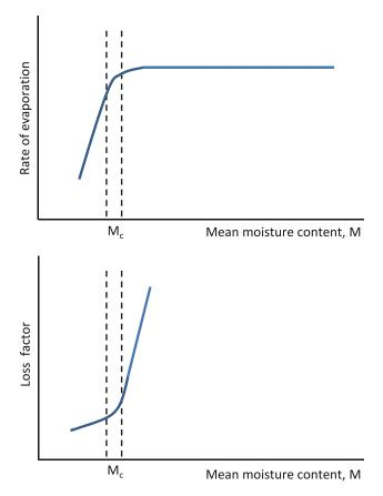
Fig. 2 Moisture content dependency of dielectric properties [66]
