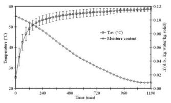
Fig. 7 Drying curve and average sample surface temperatures  $(T_{av})$  measured by thermal imaging when subjected into hot air (60 °C) drying
