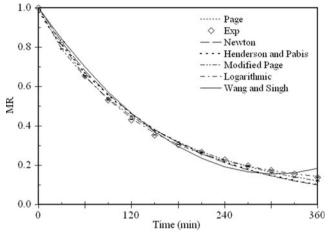
**Fig. 9** Drying kinetics of macadamia nuts when subjected into hot air (50 °C) assisted radio frequency (gap of 15.5 cm) drying simulated by six representative models against experimental values (*Exp*)
