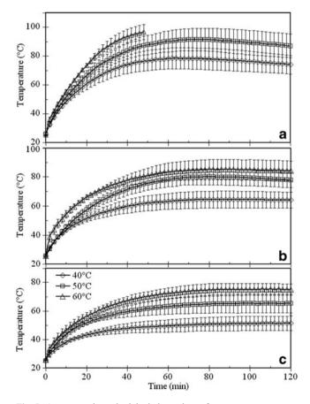
Fig. 5 Average and standard deviation values of nut temperatures over seven locations with electrode gaps of 14.5 cm (a), 15.5 cm (b), and 16.5 cm (c) and when subjected to hot air (40, 50, and 60  $^{\circ}$ C) assisted radio frequency drying
