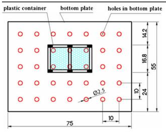
Fig. 3 Hot air inlet distributions on the bottom plate electrode and the location of the plastic container (all dimensions are in centimeters)
