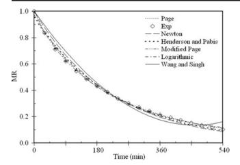
Fig. 8 Hot air drying kinetics of macadamia nuts at 60  $^{\circ}$ C fitted with six representative models against experimental values (*Exp*)
