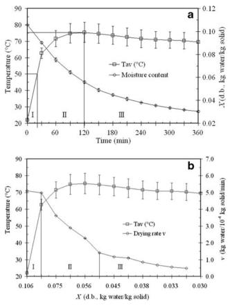
**Fig. 6** Drying curve (**a**) and rate (**b**) at three stages (I, II and III) with average sample surface temperatures  $(T_{av})$  measured by thermal imaging when subjected to hot air (50 °C) assisted radio frequency drying with an electrode gap of 15.5 cm
