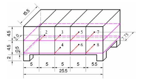
Fig. 2 The plastic container with seven fiber optic probe positions for sample temperature measurements (all dimensions are in centimeters)
