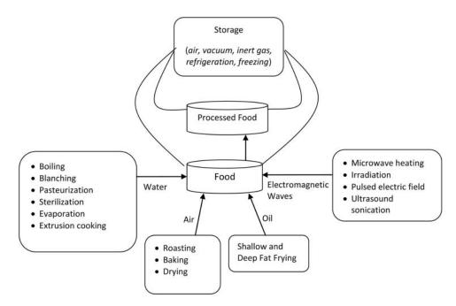
Figure 6 Heating/energy-transfer medium in various processing methods.
