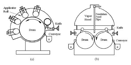
Fig. 1 (a) Single drum dryer and (b) double drum dryer.
