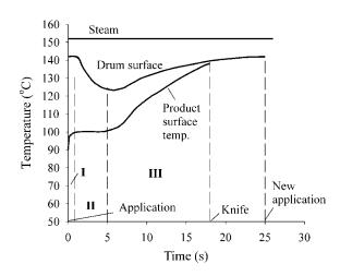
**Fig. 3** Product and drum surface temperatures during one revolution of drum drying in three different drying periods. (From Ref. 5.)
