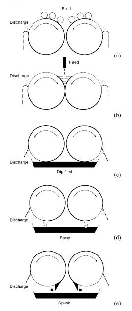
**Fig. 2** Feeding methods used in drum dryers: (a) roll feed; (b) nip feed; (c) dip feed; (d) spray; and (e) splash.
