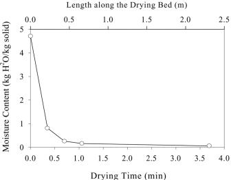
FIG. 4. Typical product residence time during RW drying of strawberry puree using process water temperature at  $95^{\circ}$ C and puree thickness of about 1.0 mm (From Ref. 46).
