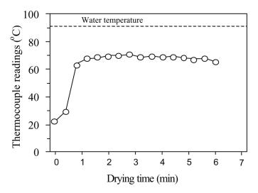
FIG. 6. Typical temperature profile for puree of thickness 0.7-1.0 mm during RW drying with the belt stationary (from Nindo et al.<sup>[47]</sup>).
