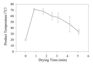
FIG. 5. Typical temperature profile for puree of thickness 0.7-1.0 mm during RW drying on a moving belt. Process water was regulated at 95°C (from Abonyi et al.<sup>[46]</sup>).
