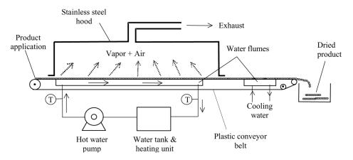
FIG. 2. Schematic diagram of Refractance Window<sup>®</sup> drying system (from Nindo et al.<sup>[47]</sup>).
