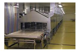
FIG. 1. Model 5 Refractance Window<sup>®</sup> dryer.
