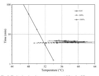
Fig. 3. Final walnut kernel temperatures (mean  $\pm$  S.D.) after RF treatments related to insect mortality as determined by thermal-death-time (TDT) curve for complete kill of 600 fifth-instar navel orangeworm larvae obtained in a heating block system (Wang et al., 2002b).
