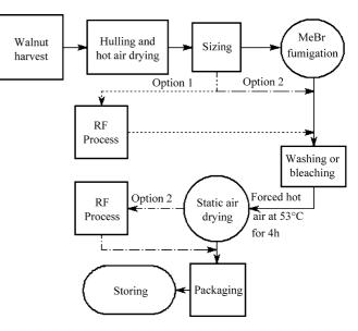
Fig. 1. Two options for placement of RF treatment in place of fumigation treatment to control pests in in-shell walnuts during industrial processes.
