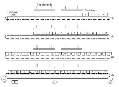
Fig. 2. Arrangement of containers during RF treatments: (a) beginning of treatment, (b) point where current is stabilized, (c) RF cavity fully loaded, and (d) containers placed back in RF system to finish treatment. Only containers 9 and 12 (shaded) were used for efficacy and quality evaluations.
