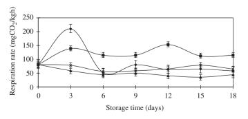
Fig. 4. Respiration rate of asparagus spears during storage at 4 °C and 90% RH after the four treatments: ( $\times$ ) CAT; ( $\blacklozenge$ ) RCS; ( $\blacksquare$ ) MAP; ( $\blacktriangle$ ) compressed Ar and Xe mix at 2:9 partial pressure [CNG]. The mean and standard deviation values were obtained by three replicates.
