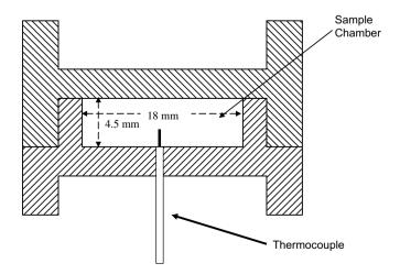
Fig. 1. Schematic diagram of aluminium TDT disk. Two halves are screwed together with an o-ring to provide a hermetic seal.
