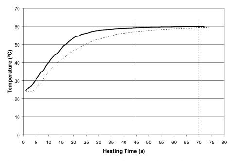
Fig. 2. A typical come-up time of liquid egg sample in a water bath at 60 °C. Solid line: Sample in a TDT disk; Dotted line: Sample in a glass tube (1 ml in 10 ml tube). The vertical lines represent the end of come-up time. The come-up time was determined when the center temperature of sample reached to 59.4 °C (99% of target temperature).
