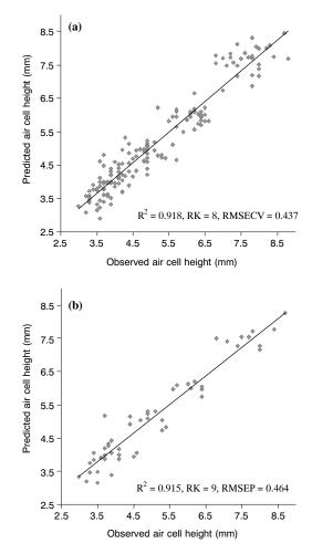
Figure 11. Observed vs. predicted values of air cell height for (a) cross-validation and (b) test-set validation using loss factor ( $\epsilon''$ ) spectra (spectra are from the average of points 1 and 2 and the 10 to 700 MHz frequency band).
