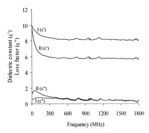
Figure 4. Dielectric constant ( $\epsilon'$ ) and loss factor ( $\epsilon''$ ) spectra for measurements at different points on shell eggs (average values for five storage durations and 35 eggs each): I = average of points 1 and 2 (opposite sides of eggs), and II = point 3 (corresponding with the air cell).
