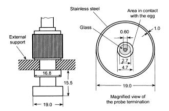
Figure 1. Schematic diagram of open-ended coaxial probe (all dimensions in mm).
