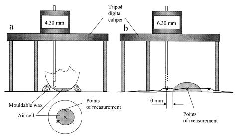
Figure 3. Methods to measure (a) the height of the air cell and (b) the thick albumen.
