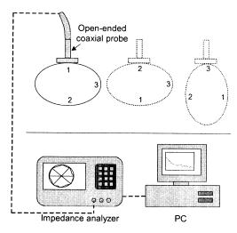
Figure 2. Measurement points on egg and experimental layout.
