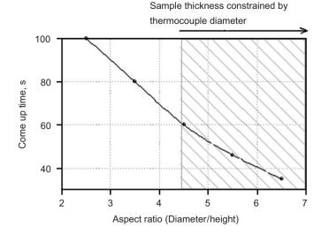
Fig. 3. Simulated effect of the aspect ratio (diameter/height of the sample cavity) on come-up time for the 1 ml disk cavity of a test cell with a 2 mm wall thickness.
