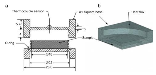
Fig. 2. Schematic representation of a test cell with a 1 ml disk cavity (A) of 18 mm diameter and 4 mm height, and finite element mesh on the top half of one quadrant (B).
