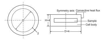
Fig. 1. Schematic representation of a disk-shaped test cell (*H*: height, *D*: diameter in mm).
