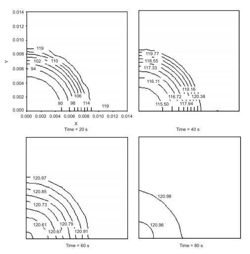
Fig. 5. Simulated temperature contour plot of a central cross-section of mashed potato sample and test cell after 20, 40, 60, and 80 s immersion in a 121  $^{\circ}$ C oil bath.
