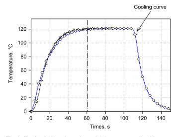
Fig. 4. Simulated ( $\triangle$ ) and experimental ( $\bigcirc$ ) temperature–time history at the center of a mashed potato sample sealed in a test cell, which was immersed in a 121 °C oil bath.
