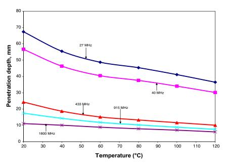
Fig. 8. Penetration depth of pink salmon anterior parts at temperatures from 20 to 120 °C (Triplicate measurements).
