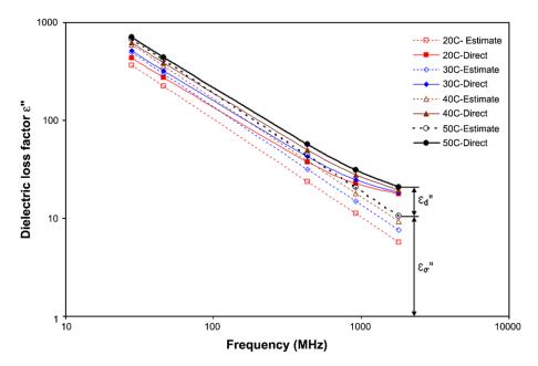
Fig. 7. Measured  $\varepsilon''$  and estimated  $\varepsilon''_{\sigma}$  of salmon fillet as a function of frequency at 20–50 °C.
