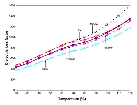
Fig. 5. Dielectric loss factor of pink salmon at four positions as a function of temperature at 27 MHz.
