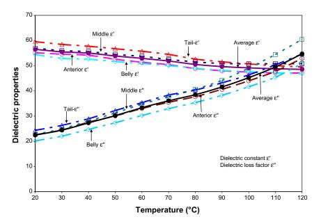
Fig. 6. Temperature dependence of dielectric properties of pink salmon at four positions at 915 MHz.
