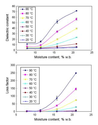
Fig. 3 – Moisture and temperature dependence of the dielectric properties of compressed chickpea flour samples at 27 MHz.
