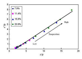
Fig. 4 – Complex-plane plot of chickpea flour samples of four moisture contents at 20–90 °C and 1.8 GHz,  $R^2 = 0.995$ .
