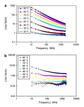
Fig. 2 – The log-log plot of the frequency dependence of the loss factor of 20.9% (a) and 7.9% (b) moisture content chickpea flour sample.
