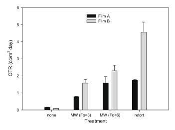
**Fig. 2.** Initial post-processing oxygen transmission rate of film A and B as influenced by microwave and pressurized hot water treatments.
