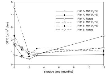
**Fig. 4.** Oxygen transmission rate of film A and B after microwave and retort processes for  $F_0 = 3$  min during storage of mashed potato at 20 °C.
