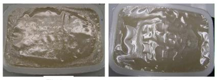
Film A Film B **Fig. 3.** Visual damage on film A and B after  $F_0 = 3$  min retort treatment.
