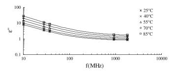
Fig. 5. Values of bread loss factor at five temperatures and 37.1% moisture content.
