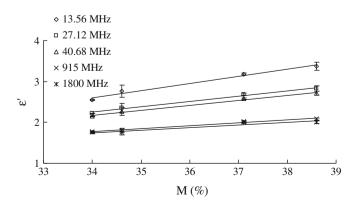
Fig. 6. Moisture content dependency of bread dielectric constant at five frequencies and 25  $^{\circ}\text{C}.$
