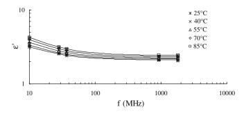
Fig. 4. Values of bread dielectric constant at five temperatures and 37.1% moisture content.
