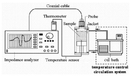
Fig. 1. Schematic diagram of the dielectric properties measurement system (Wang et al., 2005).
