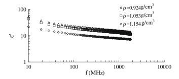
Fig. 2. Dielectric constants of compressed white bread samples with 37.1% moisture content at three densities and 23 °C.
