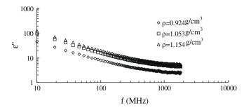
Fig. 3. Dielectric loss factors of compressed white bread samples with 37.1% moisture content at three densities and 23  $^\circ\text{C}.$
