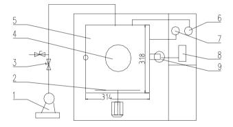
**Figure 3** Schematic of the microwave vacuum dryer. 1. vacuum pump 2. rotating tray 3. valve 4. observation window 5. drying chamber 6. infrared thermometer 7. vacuum gauge 8. magnetron power control unit 9. magnetron.
