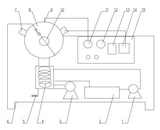
**Figure 2** Schematic of the microwave freeze dryer. 1. refrigerator 2. cooler 3. vacuum pump 4. cold trap 5. blowdown valve 6. equipment support 7. magnetron 8. drying cavity 9. infrared thermoscope 10. observation window 11. thermometer 12. pressure detector 13. PLC controller 14. power regulator 15. control box.
