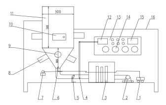
**Figure 1** Schematic of the microwave spouted dryer (dimension in mm). 1. air compressor 2. blower 3. electric heating 4. pressure detector 5.valve 6. nozzle 7. peristaltic pump 8. magnetron 9. observation window 10. operation door 11. spouted bed 12. air flow detector 13. control box 14. power regulator 15. optical fibre measurement 16. equipment support.
