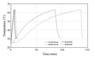
**Fig. 4.** Typical temperature–time histories of in-shell and shelled almonds in the center of a 10 cm thick container in hot air heating at 63 °C as compared with stationary hot air assisted RF heating of shelled (gap = 11 cm) and in-shell (gap = 12 cm) almonds followed by forced room air cooling in single layer samples.
