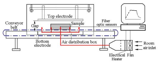
Fig. 1. Schematic view of the pilot-scale 6 kW, 27.12 MHz radio frequency (RF) unit showing the two-pair plate electrodes, conveyor belt and the hot air system (Wang et al., 2010).
