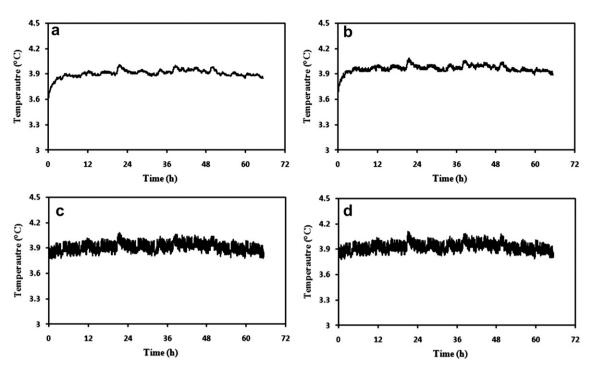
Fig. 5 – Temperature variation measured by four thermistor sensors at the set point temperature of 4 °C and 6.7 kPa pressure with 0.1 volumes  $h^{-1}$  air exchange rate in one hypobaric chamber, (a) Wet-bulb temperature; (b) Dry-bulb temperature; (c) interior chamber wall temperature; (d) exterior chamber wall temperature.
