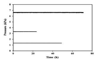
Fig. 6 – Stability of different pressures (1.3, 3.3, and 6.7 kPa) in the hypobaric chamber at 4  $^{\circ}$ C with the air exchange rate of 1, 0.2, and 0.1 volumes  $h^{-1}$ , respectively.
