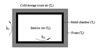
Fig. 2 – Diagram of the heat transfer model in an insulated metal chamber in a cold storage room ( $h_1$  – external surface air convection coefficient,  $h_2$  – internal surface air convention coefficient).
