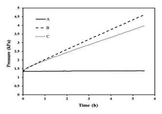
Fig. 9 – The leakage rates of hypobaric chamber under three different conditions at the temperature of 4 °C (A: Chamber only; B: With air exchange rate of 1 volumes  $h^{-1}$ ; C: With vacuum system).
