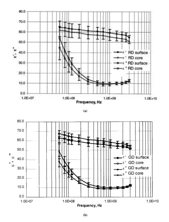
Figure 1–Dielectric constant ( $\epsilon'$ ) and loss factor ( $\epsilon''$ ) of old (a) 'Red Delicious' (RD) and (b) 'Golden Delicious' (GD) apples close to the surface and core pulp section. Error bars are standard deviations from replicates.  $\epsilon'$  = dielectric constant;  $\epsilon''$  = loss factor.
