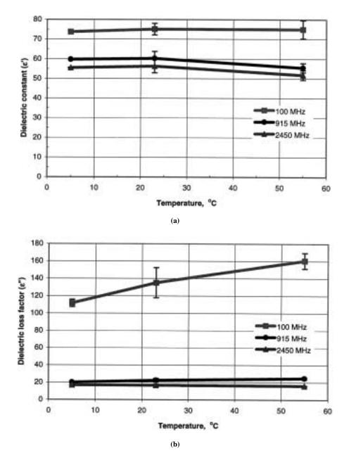
Figure 5–Effect of temperature on the dielectric properties of codling moth larvae at one RF (100 MHz) and two microwave frequencies (915 and 2450 MHz) at 23°C (a) dielectric constant ( $\epsilon'$ ) and (b) dielectric loss factor ( $\epsilon''$ ).
