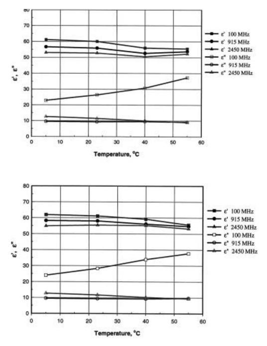
Figure 3-Effect of temperature at given frequencies on the dielectric properties of new (a) GD and (b) 'Fuji' apple pulp. Data plotted are the mean of surface and core sections.
