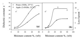
Figure 5. Comparison of dielectric properties of Red Delicious apples obtained in this study with those of potatoes reported by Mudgett et al. (1980).
