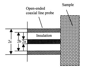
Figure 1. The open-ended coaxial line probe configuration (a = 0.45 mm, b = 1.4 mm, and c = 2.4 mm).
