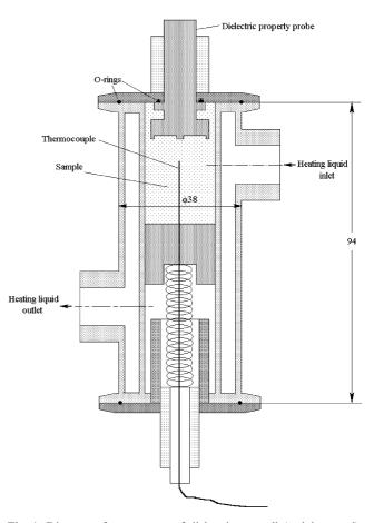
Fig. 1. Diagram of pressure-proof dielectric test cell (stainless steel), dimensions in mm.
